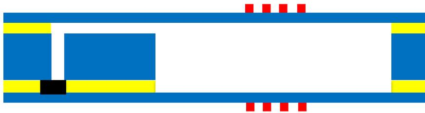
Cell with patterned transparent ITO heaters in one or both windows which drive Cs droplet condensation towards the cell sidewalls
