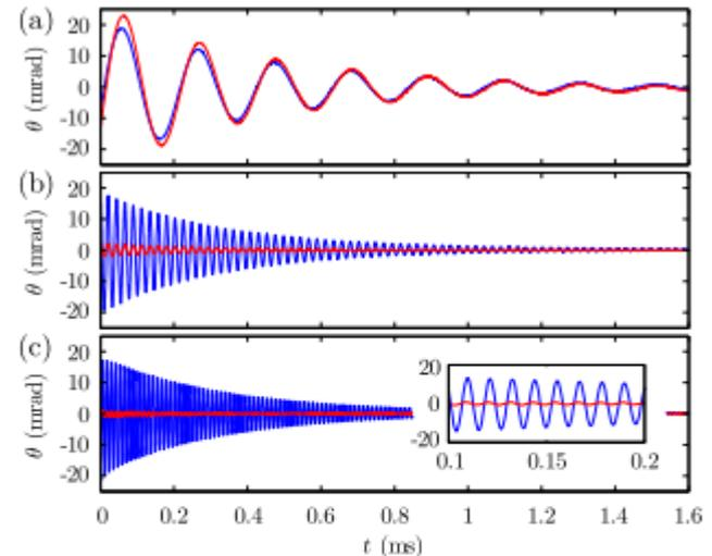
FIG. 5. Optical rotation signal (raw data) observed using single-pulse (red) and synchronous (blue) optical pumping for bias fields of (a)  $1.5 \mu\text{T}$ , (b)  $10 \mu\text{T}$ , and (c)  $25 \mu\text{T}$ . The inset in plot (c) shows  $100 \mu\text{s}$  of data to adequately resolve the oscillations resulting from the precessing atomic spins. The total measurement period was set to  $T = 2 \text{ ms}$  showing the full decay of the atomic spin polarization to equilibrium.
