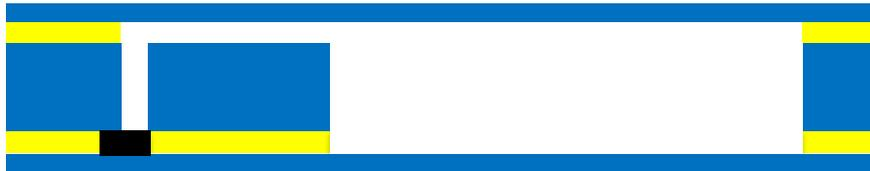
Cell with  $\text{CsN}_3$  or Cs pill reservoir. Longer optical path length set by 5 mm BF33 glass wfr with cavities fabricated by water jetting
